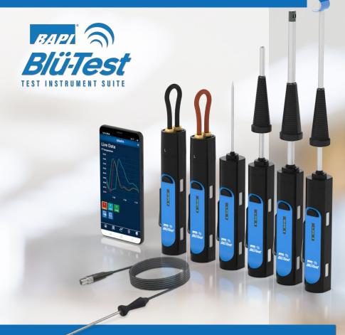
Blü-Test is a suite of NIST-traceable test instruments with onboard data logging and Bluetooth communication with Android or iOS smart devices. The suite includes multiple probes for temperature, relative humidity and differential air pressure. The Blü-Test app is available from Google Play™ or the App Store® and features logging, trending and easy sharing of files.
